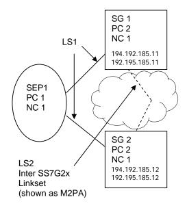
On Signaling Gateway 1, configure the IP addresses as follows and restart:
